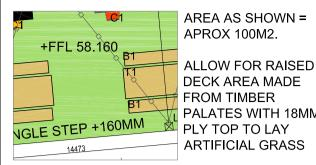
DECK AREA MADE FROM TIMBER PALATES WITH 18MM PLY TOP TO LAY ARTIFICIAL GRASS
